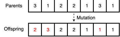
Fig. 3: An example of mutation, where the altering probability is set to C/m ( C=3 , m=7 ). The first, second, and sixth elements are mutated (marked in red).
